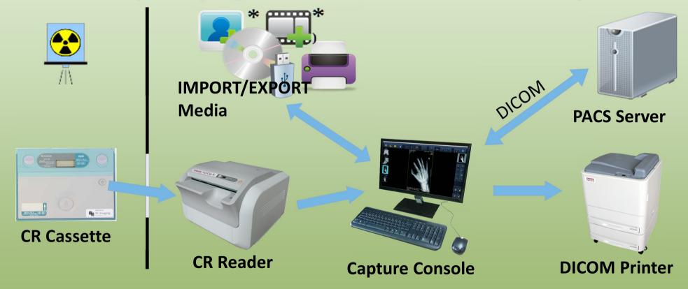
**cost effectively** converting existing Analogue x-ray Film Systems into high quality **Digital X-Ray Imaging** for general radiographic applications.
